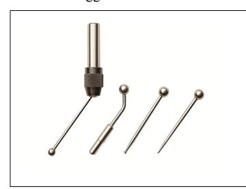
The Wiggler and Centre Finder Set is suitable for use in vertical milling and drilling machines and provides a fast and accurate method of positioning the machine spindle in the required position above the work piece.
