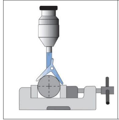
Place Centre Finder in drill chuck or collet located in machine spindle
