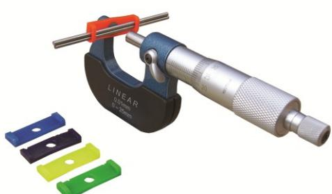
Select the correct set of wires to suit the thread to be measured
