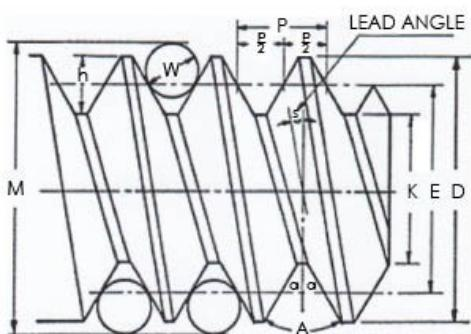
M Measurement over wires
